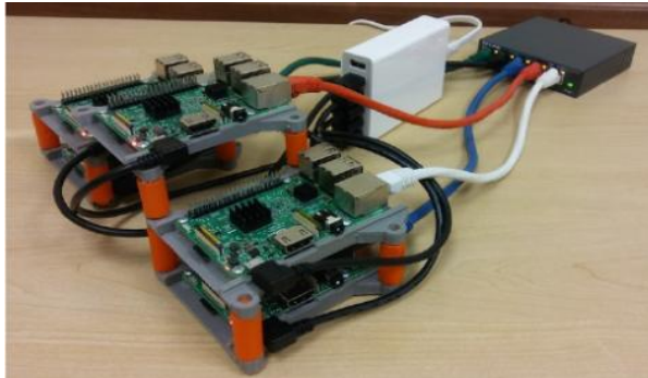
Fig. 6. Ethernet Based Raspberry Pi Cluster
