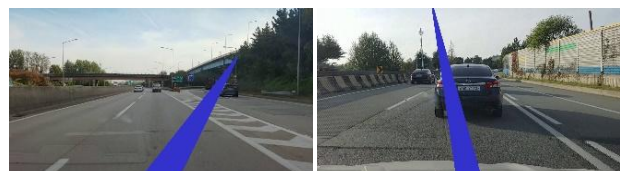
Fig. 24. Lane detection failure image visualization
