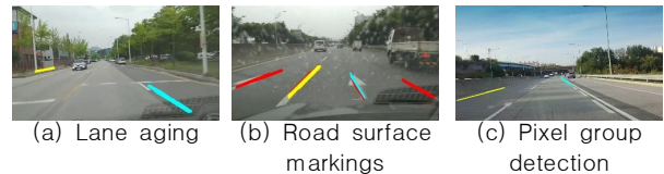
Fig. 13. Lane detection failure result
