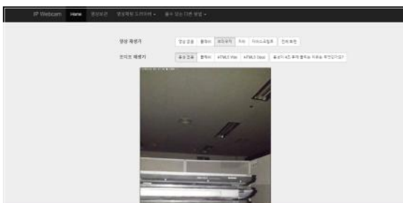
Fig. 7. Access to Domestic IP Camera without Authentication
