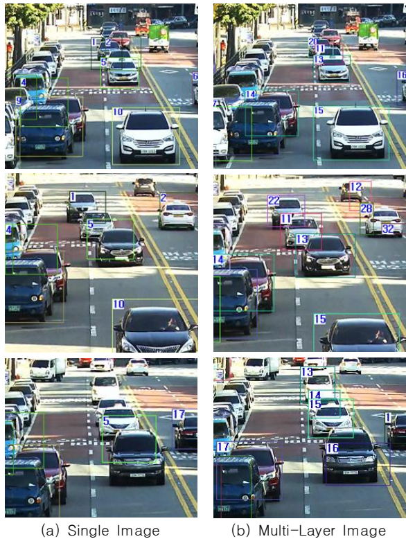
Fig. 12. Detection result for small dense vehicle
