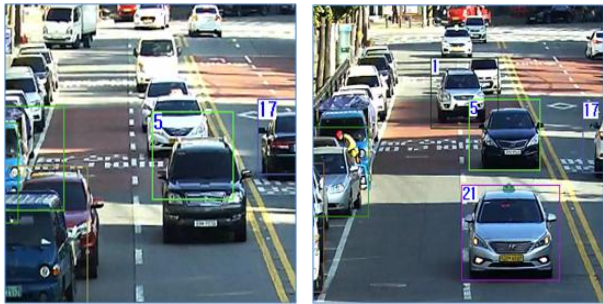
Fig. 6. Detection Result in Small Dense Vehicles case
