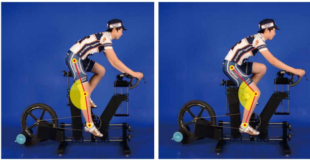
Fig. 11. The height of the saddle and the angle of the knee
