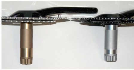
Fig. 21. Length of crank shaft[11]
