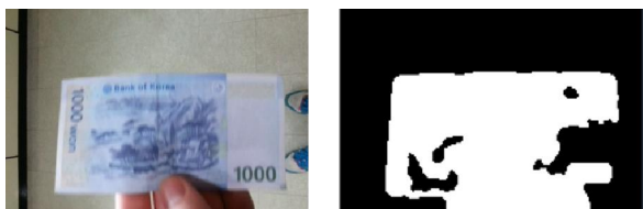
Fig. 4. Input video frame (left) and its corresponding foreground binary matrix (right)
