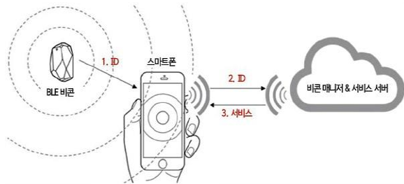
Fig. 2. concept of BLE(Bluetooth Low Energy) Service
