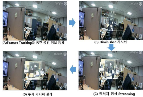
Fig. 3. Process of the proposed transparent telepresence visualization (A) Registration specific area using feature tracking methods (B) Visualization of the diminished reality through destruction effects (C) Realtime telepresence streaming (D) Results of transparent telepresence visualization
