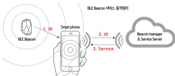
Fig. 6. Beacon operation principle[11-13]
