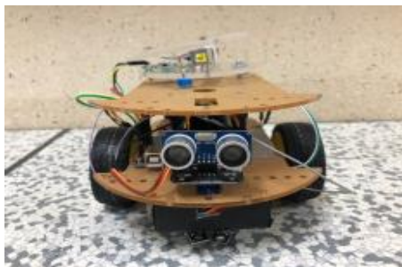
Fig. 12. Autonomous Vehicle with Ultrasonic sensor
