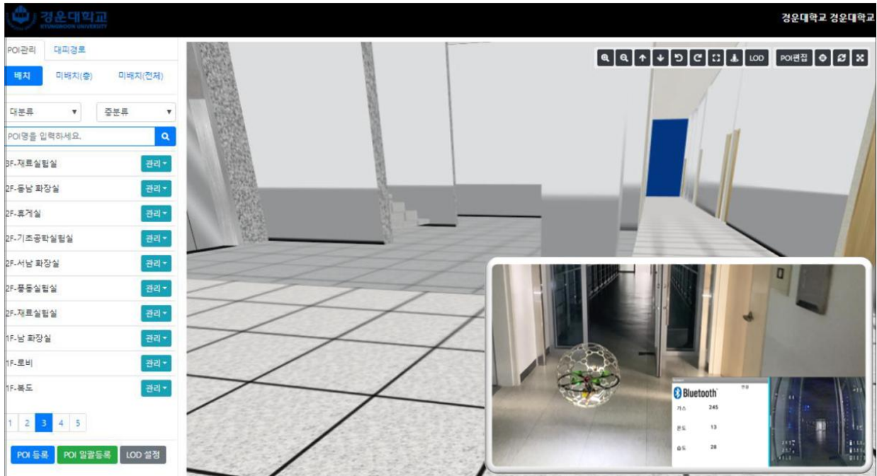
Fig. 9. Mapping of drone measurement values and video information to the existing digital twin control system (video transmitted by Sense Box)
