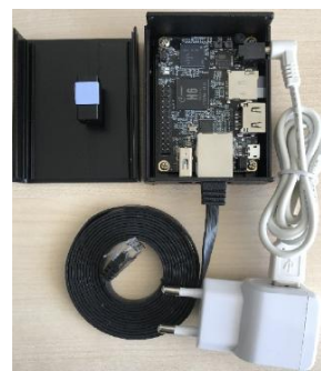
Fig. 6. Inside of Network Security Sensor of Supposed system
