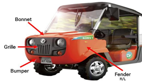
Fig. 1. Five components of the front part of an agricultural electric vehicle[9]
