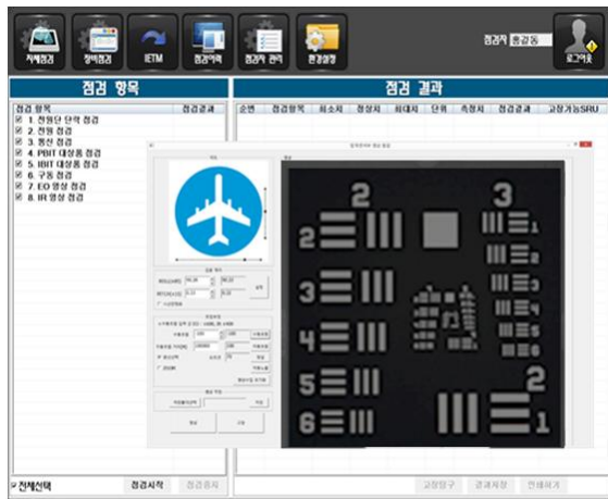
Fig. 12. EO/IR Automatic Test Software and Simulator
