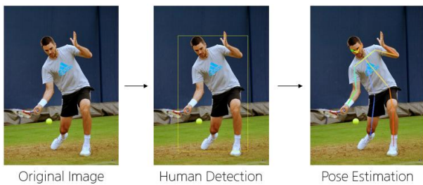
Fig. 2. Deep-Learning based Pose Estimation
