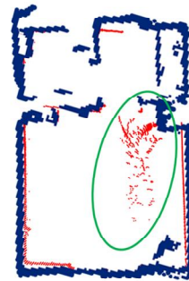
Fig. 8. The Result of 2DLiDAR scanning and Map Mergers
