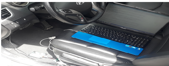
Fig. 9. Connection of development system OBD-II to passenger car
