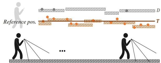
Fig. 5. Navigating reference plane ( T : search range, D : plane outside the range of T ).
