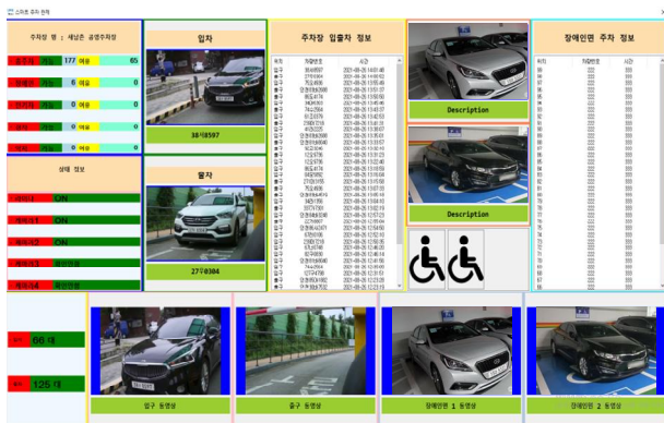
Fig. 12. Administrator UI of smart parking control system
