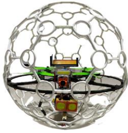
Fig. 7. Drone equipped with Air pollution measurement module
