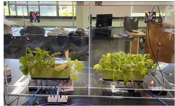
Fig. 2. Sensor cage for multi-control and control device using Arduino
