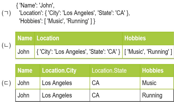
Fig. 8. Example of Flattening Operation for JSON
