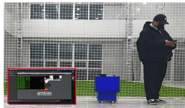
(c) Obstacle recognition test with LiDAR and ultrasonic sensor
