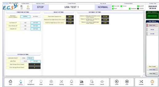
Fig. 9. Set the motor speed of clean roll
