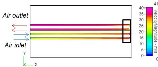
Fig. 5. Velocity at tube side of the flue gas.
