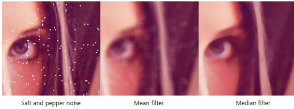
Fig. 10. Compare Mean filter and Media filter
