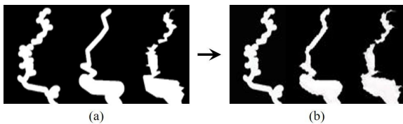
Fig. 2. Enhanced details of crack with CNN : (a) input data, (b) output data.
