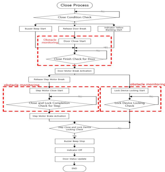
Fig. 10. Process diagram for door close.
