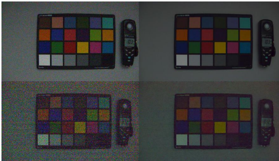
Fig. 10. Raw and sRGB colorchecker image visualized by ISP (1lux noisy, 1lux denoised, 0.1lux noisy, 0.1lux denoised from left top to right bottom)
