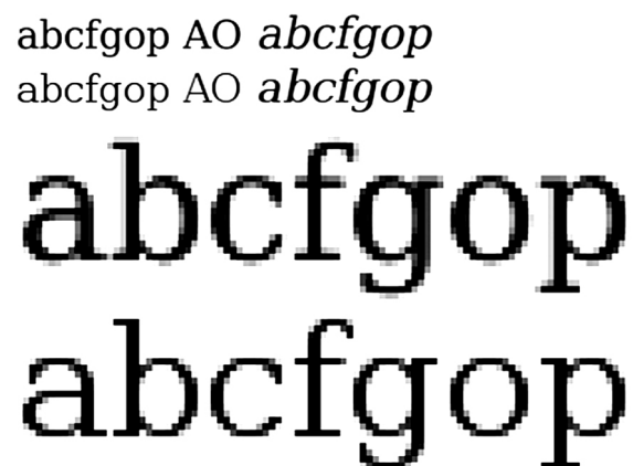
Fig. 1. A font test without hinting (upper rows) and with hinting (lower rows)
