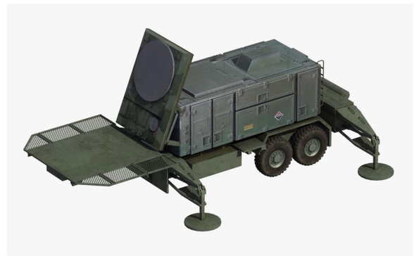
Fig. 2. Multi-function radar for vehicle of patriot missile system
