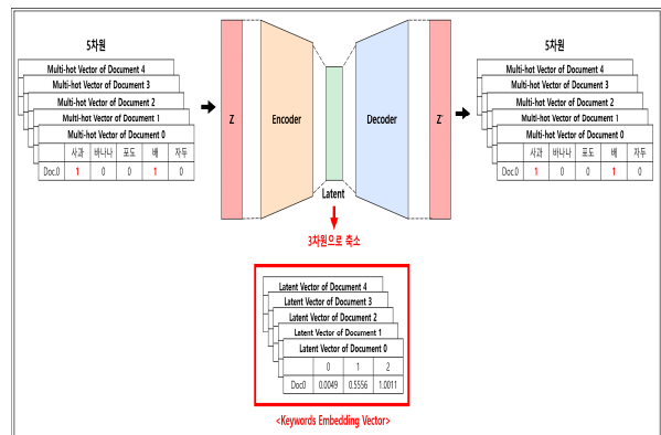
Fig. 7. Example of Latent Vector Generation
