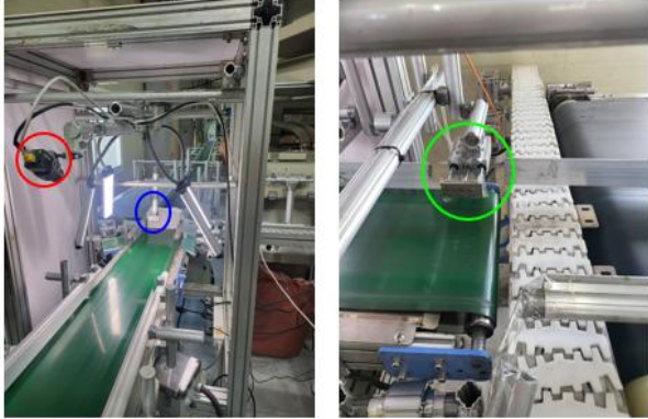
Fig. 8. Proposed vision system
