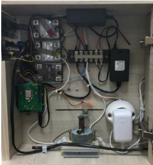
Fig. 6. Chick Incubator architecture
