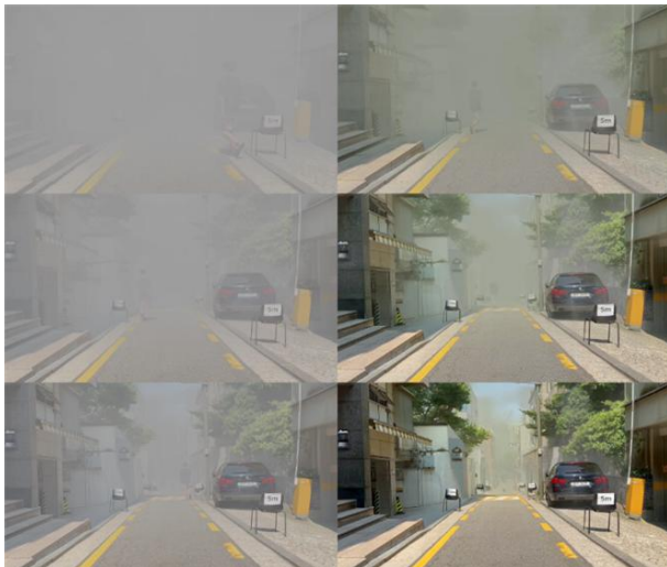
Fig. 7. The following images are from synthetic fog video (left) and defogged video (right) with visible distances of 5m, 10m, and 15m from top to bottom. These frames represent the moments when a pedestrian moves out of the visible range.
