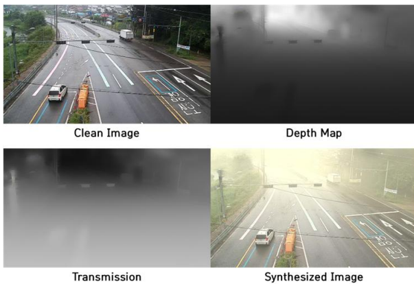
Fig. 4. Intermediate images of our fog image synthesis pipeline.
