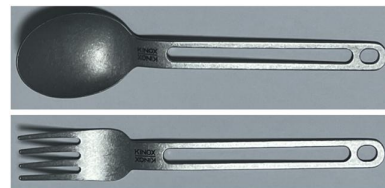
Fig. 15. Products that are labeled as STS 316 grade, but are suspected to be STS 304 grade spoon(up) and fork(down)
