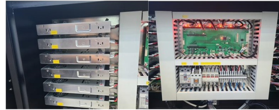
Fig. 10. Separate power supply for each axis
