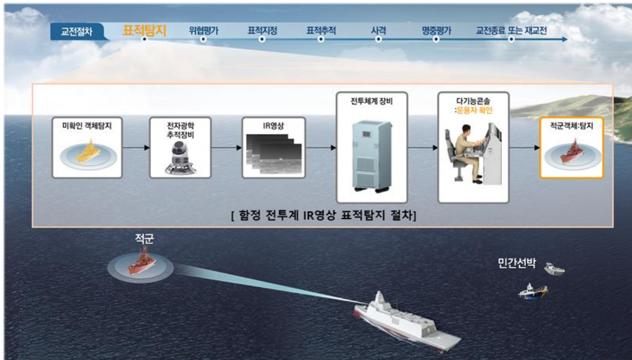
Fig. 1. The Procedure of Naval Combat Management System IR Image-based Target Detection
