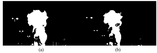
Fig. 5. The result of detecting the center of the flame as the gamma value changes : (a) \gamma=40 , (b) \gamma=150
