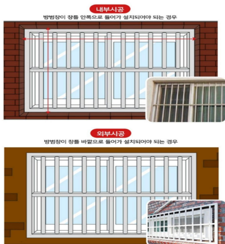
Fig. 1. Installation of general security windows
