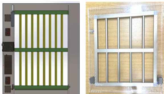
Fig. 10. Isometric drawing and actual appearance of a security window
