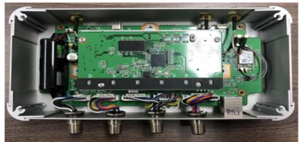
Fig. 9. Internal Diagram of RTLS/IoT Monitoring Terminal
