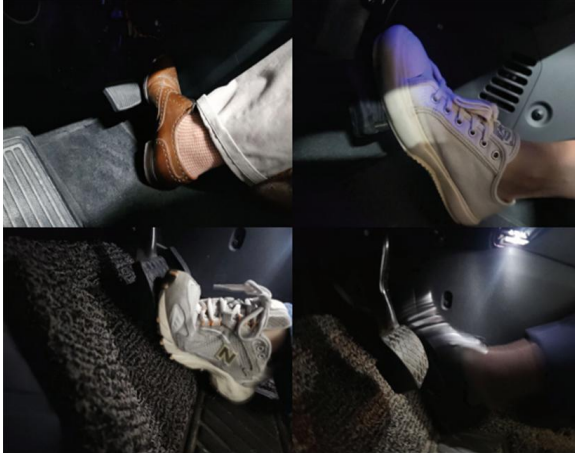
Fig. 4. Data collected from the camera for 4 pedal operation classes (clockwise from top-left): (1) No pedal operation, (2) Slight brake pedal operation, (3) Full brake-pedal operation, and (4) Accelerator pedal operation.
