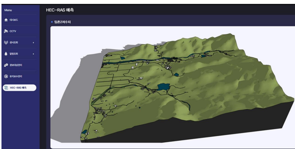
Fig. 13. 3D geometry model for flood prediction simulation
