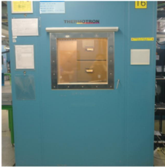
Fig. 4. Temperature and humidity test in chamber.
