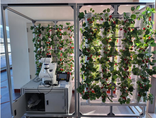
Fig. 3. Experimental setup consisting of the research vertical-farm mock-up and the robot system
