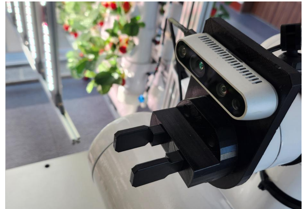
Fig. 1. RGB-D camera module(D435i) mounted on the robot
