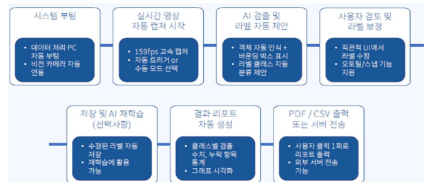
Fig. 3. Workflow of the Proposed Defect Detection Process
