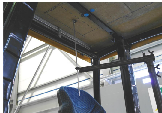
Fig. 1. FOPS deflection measurement by using a link device
