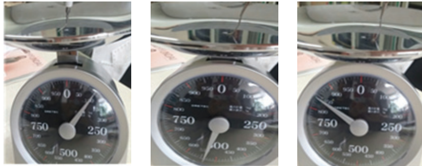
Fig. 3. Lateral pressure measurement using the weighing scales
