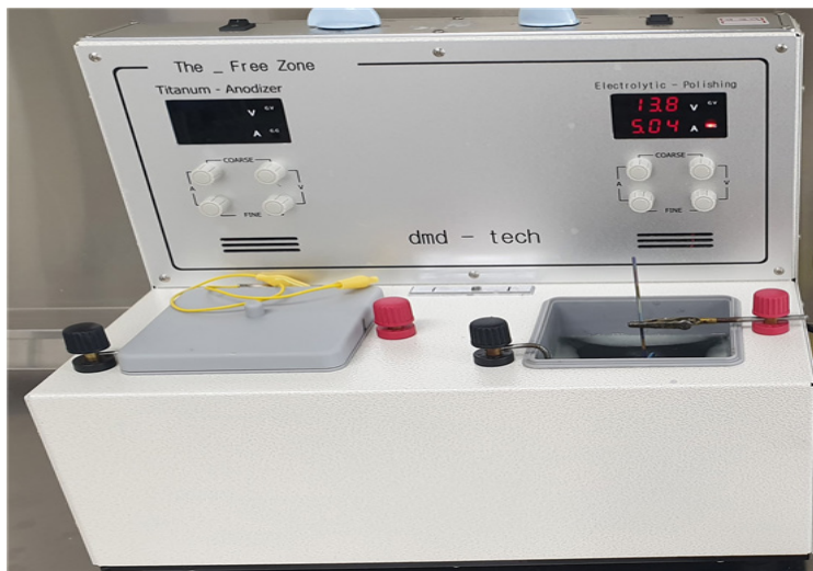
Fig. 3. Electro polisher. Dmd-tech for conducting electro polishing.
